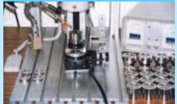
Laser welding of diaphragms.
